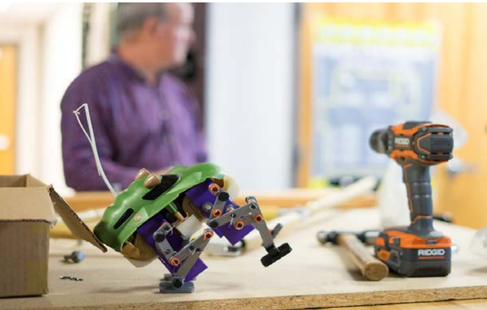
The first walking bicycle prototype designed by students was made from an electronic remote controlled car. The wheels were replaced by legs printed on a 3D printer.
